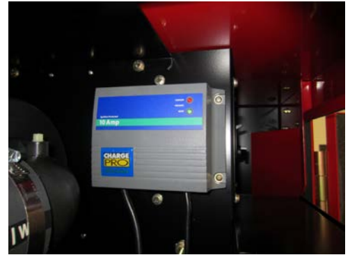
Battery chargers can be installed on all TS units. No drilling required for easy installation.
