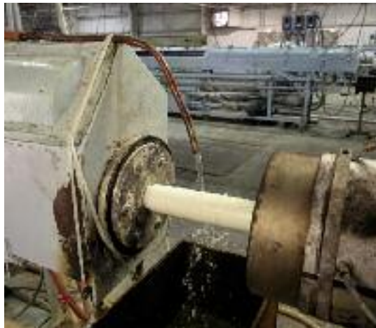
(Left) A plastics manufacturer uses vacuum during the extrusion process to rid PVS pipe of process contaminants.
