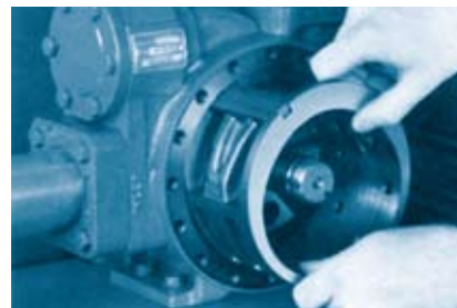
Easily replaceable liner restores efficiency.
