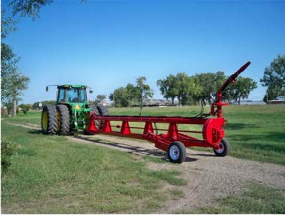
*PTO Single Wheel Axle with Nozzle Discharge*
