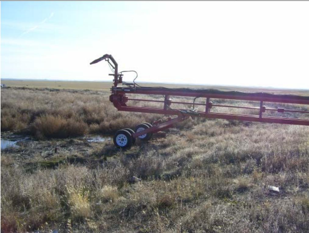
Hydraulic Double Wheel Axle with 7 foot lift
