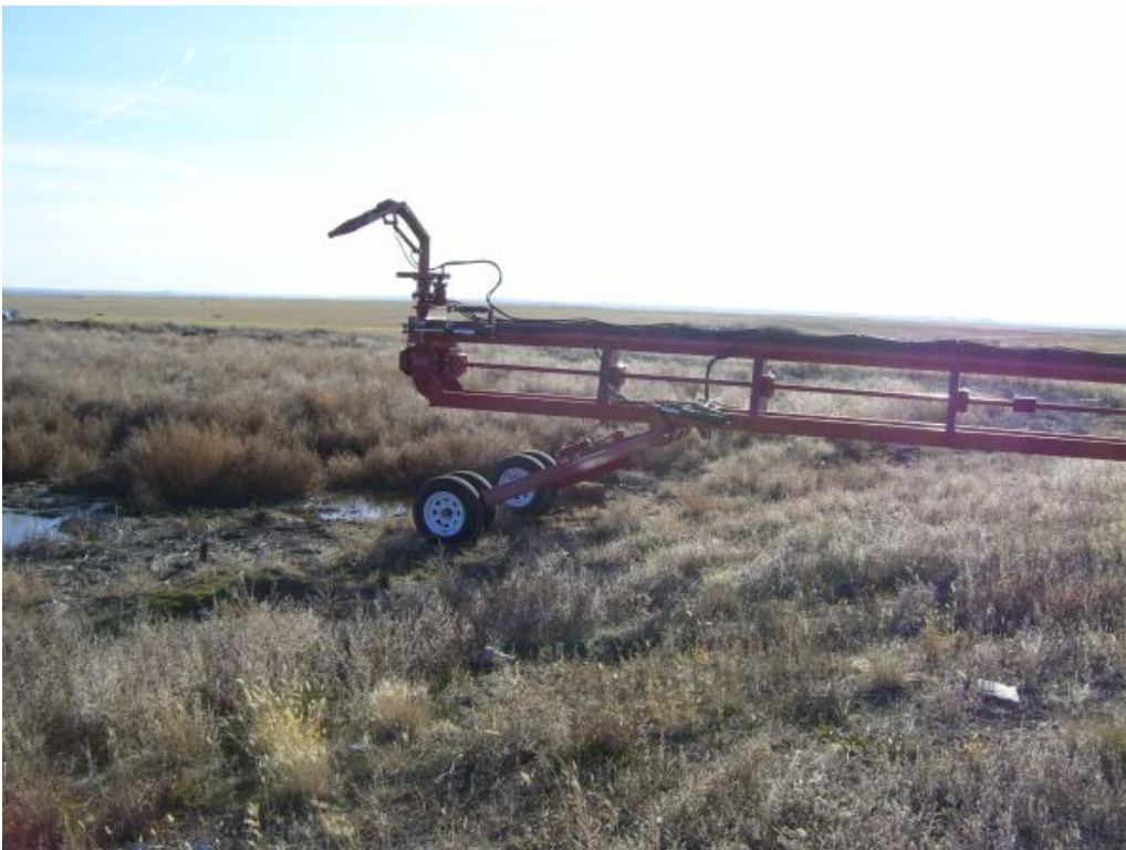
Hydraulic Double Wheel Axle with 7 foot lift
